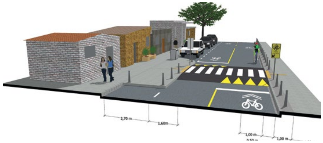
A shared bicycle street, bike boulevard design with road markings and traffic calming measures.
