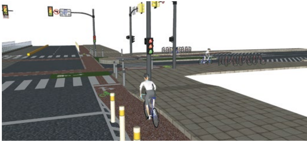
Bicycle signals can be clearly placed to inform when cyclists can cross.
