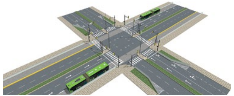
Four-way intersection with curbside bus lanes.
