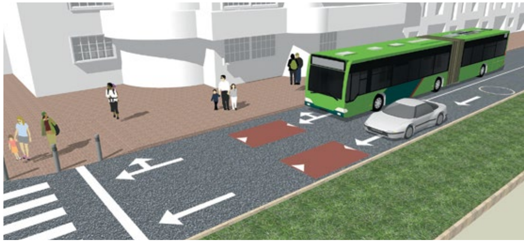
Speed cushions can allow wide-axle vehicles to pass over the cushion to increase comfort for bus passengers.
