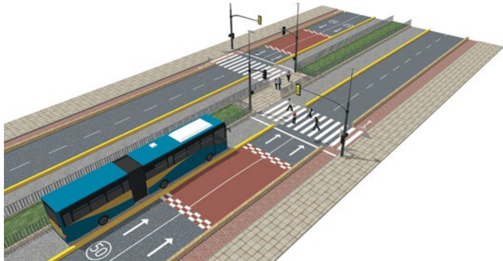
Midblock crossing on an urban arterial.
