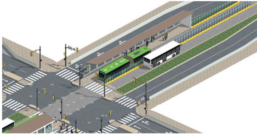
Pedestrian access to a median BRT station.
