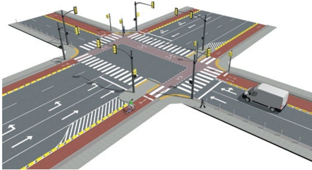
Cycle tracks separated from car traffic through physical barrier.
