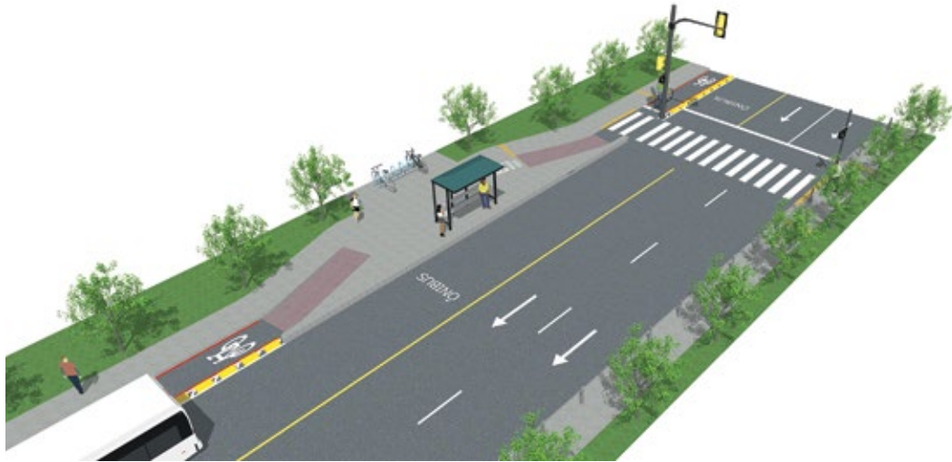
Bike path design should accommodate the needs of both bicyclists and pedestrians at a bus stop.
