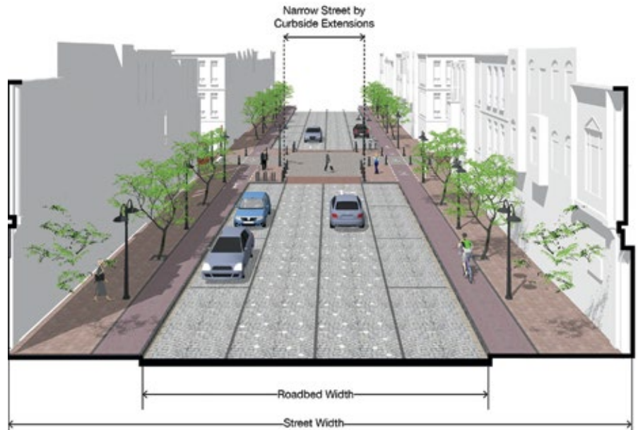
Illustration showing the different aspects of street width.
