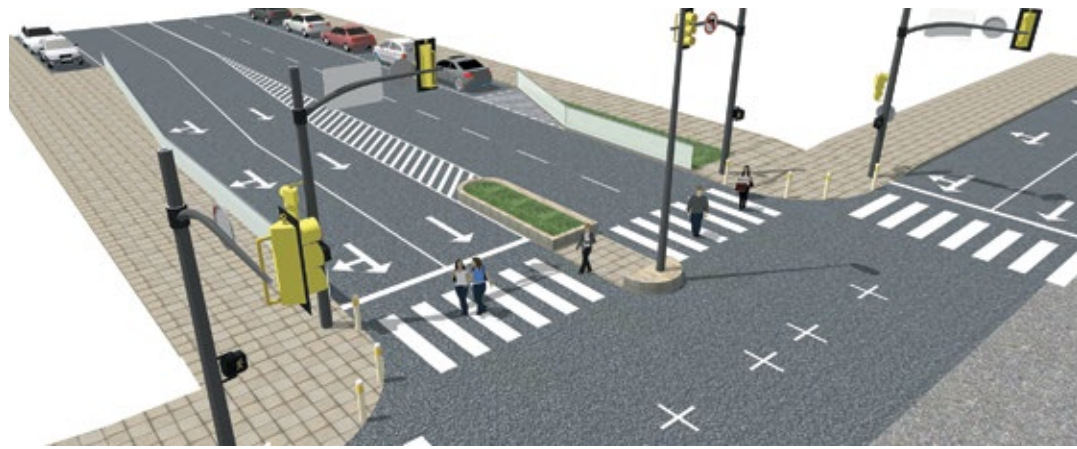
Central median refuge without a continuous median.
