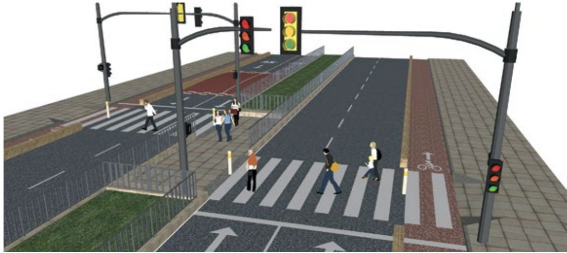
Central median refuge, seen on a 4-lane road; applicable to two-lane roads as well.
