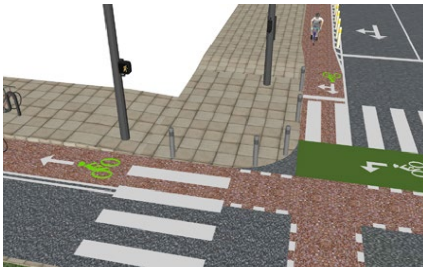
An intersection enhances the view between drivers and cyclists as they approach the intersection, and a two-step left-turn box.
