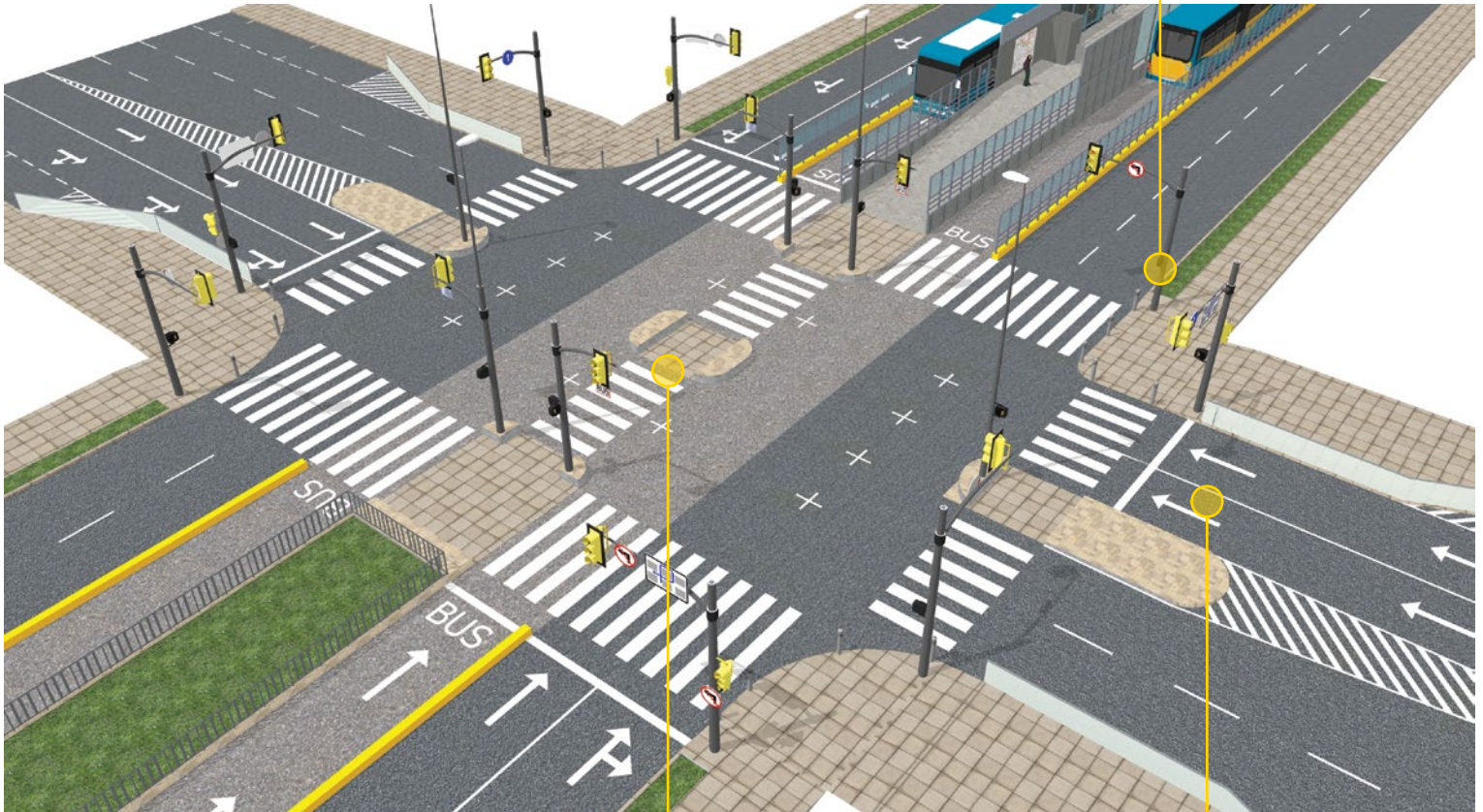
Figure 49 Station access on an urban arterial
