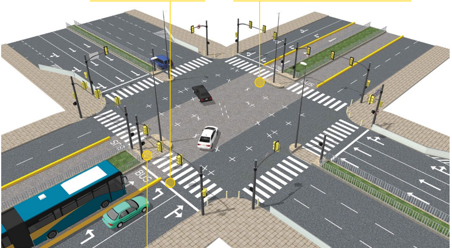
Figure 29 Major four-way intersection, with left turns
