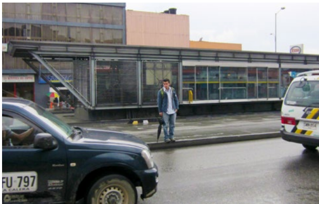
Figure 52 Pedestrian crossing the road in front of a station with no barrier between the bus lane and mixed traffic.
