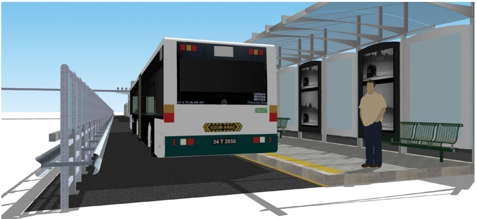
Figure 68 Design concept illustrating a combination of a double-sided crash barrier and a high guardrail, recommended for freeway-running BRTs
