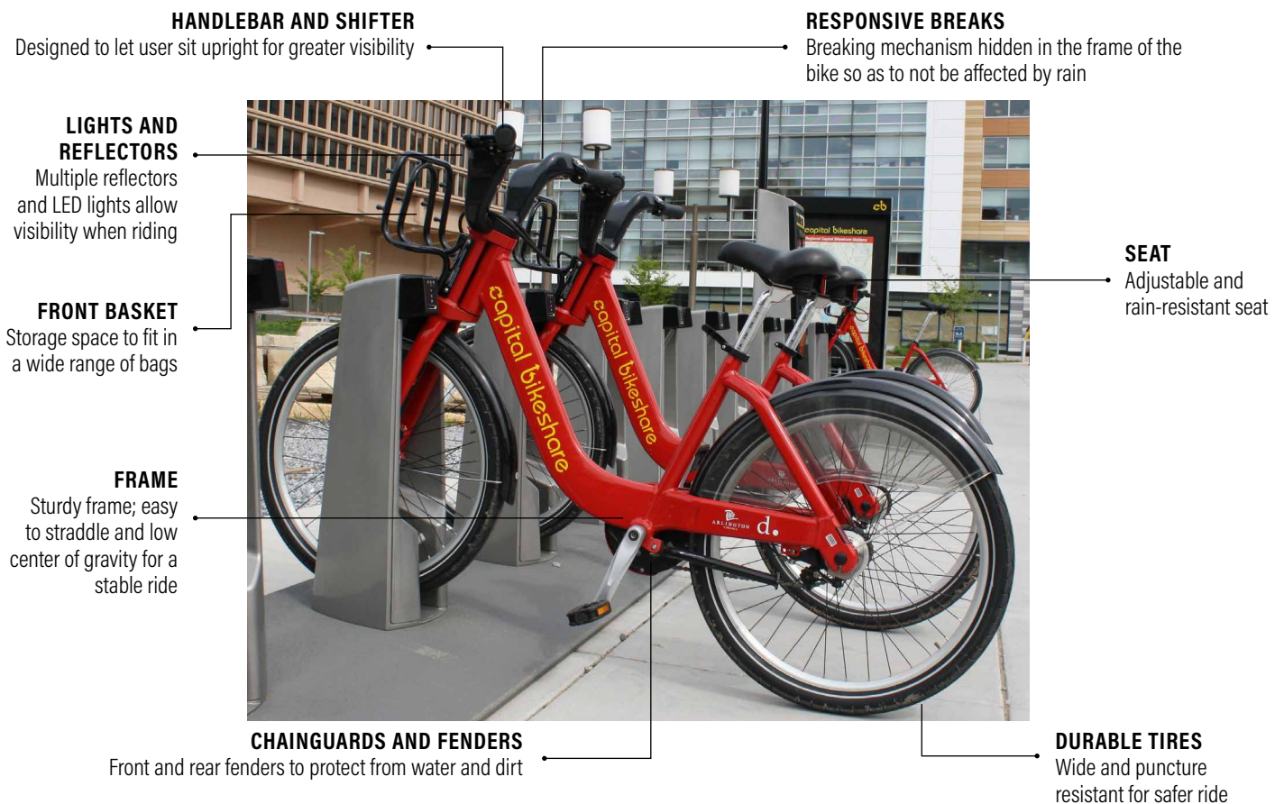
Figure 7 | Common Safety Features on Docked Bike-sharing Bicycles
